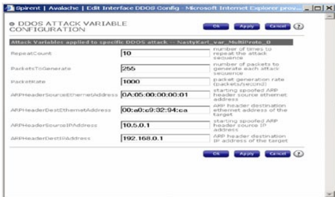
Figure 10: Example of configuring a DDoS attack using the Inline DDoS option.
