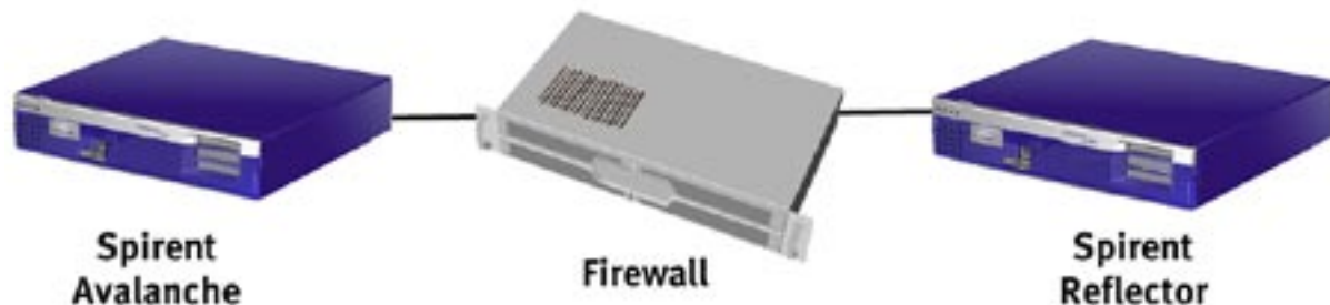
Figure 1: The most basic network testbed for testing firewall performance, with a client traffic simulator on one side and a server simulator on the other side. Firewall testbeds can become quite complicated, especially for tests that include servers and clients on both sides of the firewall and servers in the DMZ.
